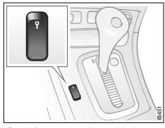
Switch for operation of central locking
