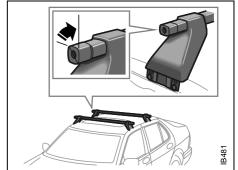
3 Start on the left-hand side of the car. Rest the carrier carefully across the roof, with the rigid foot towards you. Hold the foot clear of the roof to avoid damaging the paintwork.
