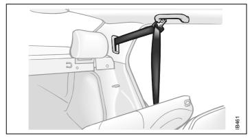
Outer safety belt hooked onto courtesy handle
