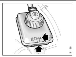
Brake and clutch-fluid reservoir
