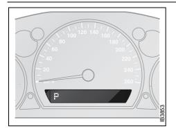
Selector-lever indicator on main instrument panel
