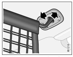
Attaching the cargo net to the roof
