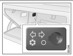
Sliding cover in glove compartment to admit cold air
