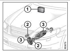
Oxygen-sensor-controlled injection system
