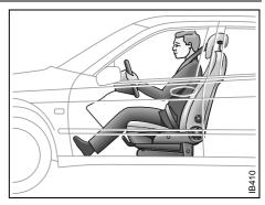
Correctly positioned safety belt
