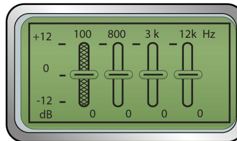
6. Scroll Select each vertical control level. Use the Scroller to move the control knob up or down to vary the amount of boost or reduction in the selected frequency range.
