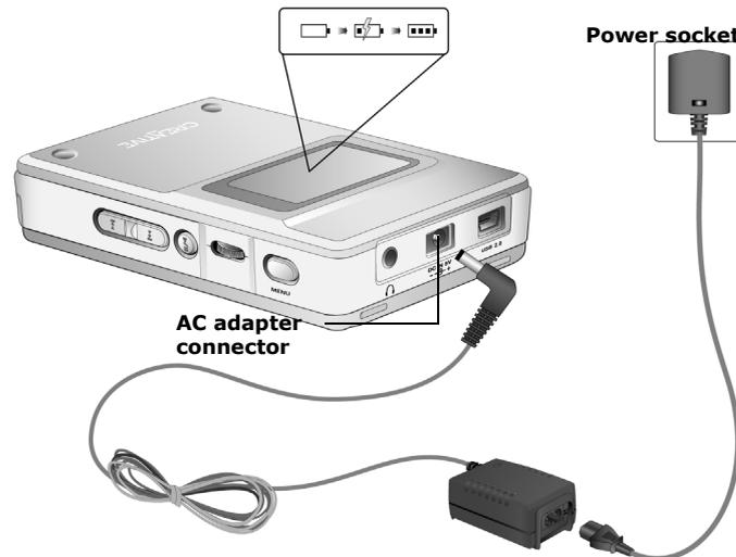
Figure 2-4: Connecting the player to a power socket.
