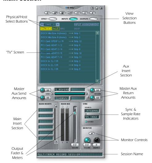
The main section contains all controls for controlling the main mix elements as well as a "TV screen" for viewing the parameters of the current selected insert.
