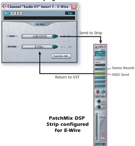
E-Wire bridges the gap between hardware I/O and the VST world. The E-Wire VST plug-in sends audio to a strip containing the desired effect. An ASIO Send routes the audio back to E-Wire VST.
