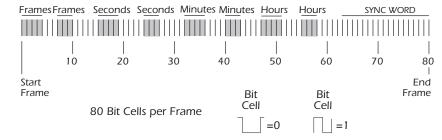
There are four types of SMPTE time code in general use: 24, 25, 30 frame-per-second and 30 drop-frame. In general, you should choose one rate (30 non-drop is common in audio) and stick with it for initial recording and later editing.
