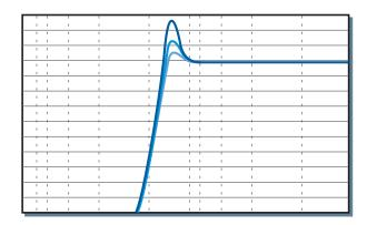
In this mode, the Highpass filter can have up to a 48dB/octave rolloff slope. The Highpass Rolloff, Highpass Frequency and Highpass Resonance parameters are available for editing the filter response.
