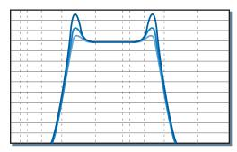
However, if the Highpass Freq parameter is greater than the Lowpass Frequency parameter, the passband effectively disappears, since the part of the spectrum which is above the highpass and below the lowpass is non-existent. As a result, you'll hear a rapidly attenuating bandpass response as the corner frequencies diverge.
