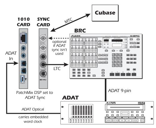
The Sync Card should not be used as both the SMPTE and word clock master. Word Clock is generated by the Digital Audio System and NOT by the software application (Cubase). SMPTE is not locked to Word Clock inside the Sync Card—they are completely independent.
