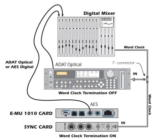
This diagram shows the proper way to connect word clock if you don't have a multi-output word clock generator. The last device in a Word Clock chain should have Termination ON.
