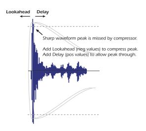
At positive values, the signal path delay is zero; instead, a delay of up to 50 milliseconds is inserted into the sidechain path containing the level detector. This delay can be used intentionally to cause the compressor to miss signal peaks, retaining the "punch" and
