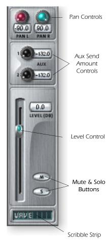
The Pan control comes before the Level Control and Aux Sends in the signal flow. On stereo strips we use an unconventional pan section with two pan pots – one for the left part of the signal and one for the right part of the signal. This feature allows you to independently position both sides of the stereo signal. A conventional stereo balance control only allows you to turn down one side or the other.
