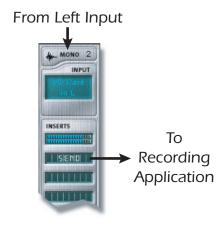
To connect an input to your recording software: **Add a Host ASIO Insert.**
