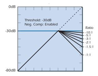
wote: You may need to use the Gain parameter to keep these restored peaks from clipping the compressor output since Auto Makeup gain doesn't automatically take the compressor tail into account.
