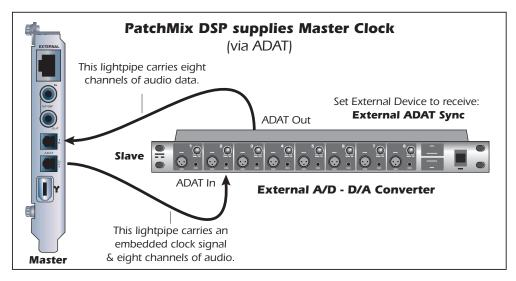
In the second example a second lightpipe is used to supply "embedded word clock", as well as eight channels of audio to the external A/D - D/A. The external device MUST be set to receive external clock via ADAT or the units will not be synchronized. The E-MU Digital Audio System is the Master and the external A/D - D/A is the Slave.
