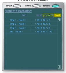
The Host Output display shows all the Insert Routings in addition to the Main Mix and Monitor out routings. Click on the desired row to make or break a physical output connection.
