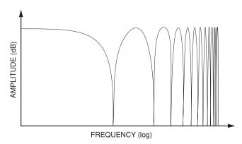
A low frequency oscillator is included to slowly change the delay time. This creates a rich, sweeping effect as the notches move up and down across the frequency range. The amount of feedback deepens the notches, intensifying the effect. You can invert the feedback signal by choosing a negative feedback value. Inverting the feedback signal creates peaks in the notch filter and deepens the effect.
