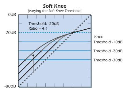
This diagram shows the effect of varying the Soft Knee Threshold. Compression is 1:1 (no compression) at the Knee Threshold and smoothly transforms into the selected compression ratio at the Compression Threshold. The upward arrow shows the additional gain added to signals below the Threshold.
