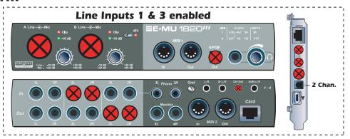
At the 176.4kHz or 192kHz sample rates, you sacrifice S/PDIF, line input 3, and line output 3. ADAT optical is reduced to two channels. You can choose one of the following options:
