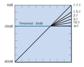
♦ Tip: A ratio of Infinity: 1 combined with high threshold and fast attack/release results in an effective peak limiter.
