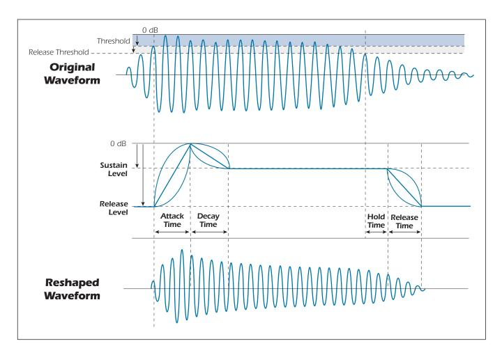
Attack, Decay and Release times are all adjustable, and the shape of each of these segments is selectable between exponential, linear, or logarithmic. An additional Hold Time can be used to extend the Sustain phase past the point where the signal has passed the Release Threshold.
