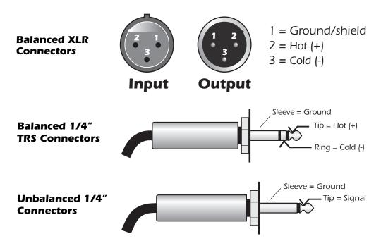
Balanced cables have one ground (shield) connection and two signal-carrying conductors of equal potential but opposite polarity. There is one "hot" or positive lead, and a "cold" or negative lead. At any point in time, both conductors are equal in voltage but opposite in polarity. Both leads may pick up interference, but because it is present both in and out of phase, this interference cancels out at the balanced input connection.
