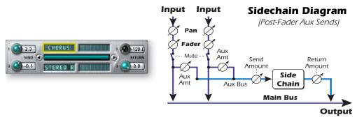
You can also use the Auxiliary Sends as two extra mix buses. By turning the Aux Return amount all the way down and dropping an Insert Send into the chain, you can send the Auxiliary bus to any output you wish. See <u>"Insert Section"</u> for more information.,
