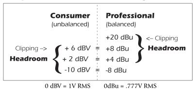
An input setting of -10 is compatible with consumer audio gear and works best with low level signals. (-10dBV is approximately 12dB lower than +4dBu.) Choose the setting that allows you to send or receive a full scale signal without clipping.
