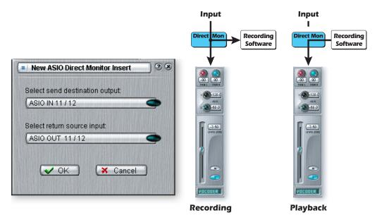
The Direct Monitor Send/Return also allows the recording application to control volume and pan. Normally when using direct monitor recording you'll want to control the volume and pan from the recording application. In this case, set the PatchMix DSP stereo pan controls hard left and right, mono pan controls to center, and the fader to OdB.
