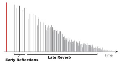
After a short pre-delay period, the echoes from the closest walls or ceiling are heard. These first echoes, or early reflections, vary greatly depending on the type of room. Some time after the early reflection cluster ends (late reverb delay), the late reverberation (a dense cloud of complex wall reflections) begins and decays according to the time set by the Decay Time parameter.
