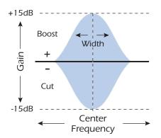
This single band parametric equalizer is useful when you just want to boost or cut a single range of frequencies. For example, if you just want to brighten up the lead vocal a bit, you might choose this EQ. This EQ offers up to  $\pm 15 dB$  cut or boost.
