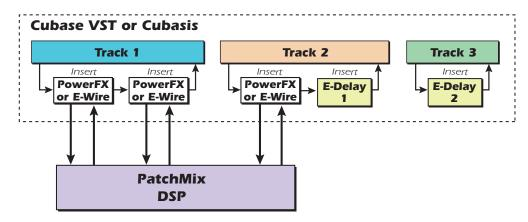
Since track 1 uses two PowerFX/E-Wire inserts, the delay of all the other tracks must equal two. Track 2 has one PowerFX/E-Wire insert and so adding one unit of E-Delay keeps it time aligned. Track 3 doesn't use a PowerFX/E-Wire insert and so it needs two E-Delay Units to remain in alignment.
