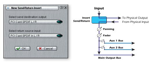
▼ If the source or destination you want to use is not available in the list, they are probably already being used elsewhere. Check the input Strips, Inserts and Output Assignments.
