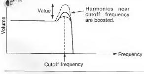
The higher the value, the higher the resonance peak and the more obvious the effect. At or near the maximum value (3 l), the VCFs go into self-oscillation, producing a pure sine wave, which can be used as an additional sound
