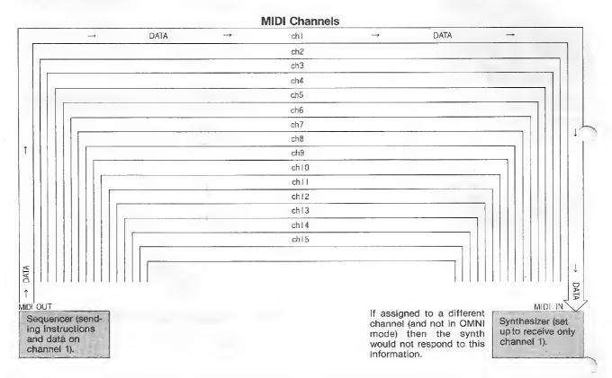
If you are using a MIDI sequencer or computer then you can assign particular instructions and data to particular channels. By assigning the various receiving synthesizers and drum machines to different channels, you can make each instrument play a different part of your musical composition. This kind of complex MIDI system is shown here.
