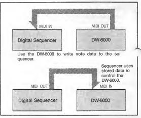
If using a digital sequencer, it is usually possible to program it in real time by simply playing on the DW-6000.
