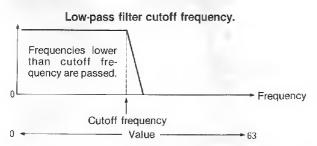
At the highest value, 53, all harmonics are passed. The lower the value, the more harmonics are cutoff, so the sound becomes progressively rounder or less bright.
