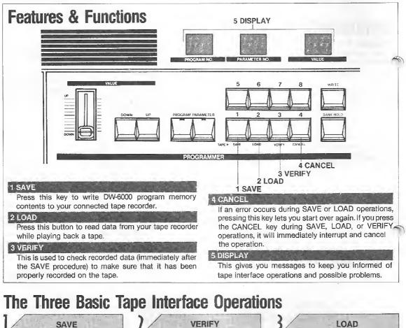
During a SAVE Operation, the DW-6000 sends all oif its stored sound program data (the parameter values for all 64 program numbers) out the TO TAPE jack on the rear panel. The connected tape recorder is used to record this data during a SAVE operation. This should always be performed immediately after a SAVE operation. VERIFY is used to check whether or not the SAVE operation has been successful. You play back the tape (through the FROM TAPE jack) that you have just SAVED the data on,
